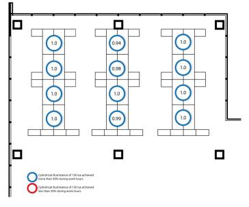
Figure 7. Cylindrical illuminance measured at occupant workstations across a one-day period, showing that sufficient lighting above 150 lux was provided well over 50% of the working period.
