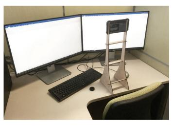
Fig. 4. Assessment of the luminous environment and glare sources using a mobile device and micro fish-eye lens.
